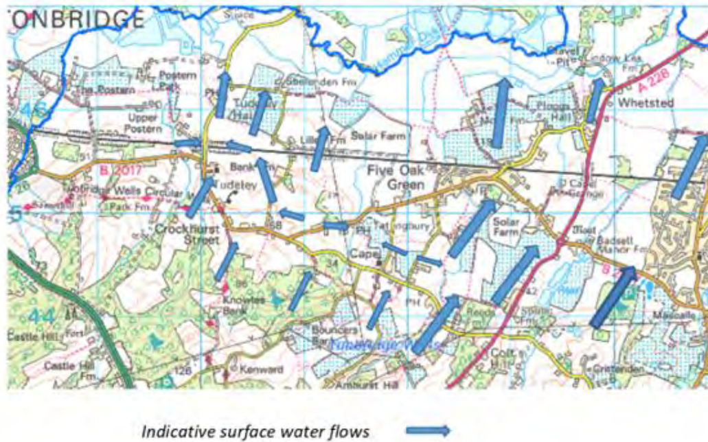
Figure 8: Indicative surface water flows in the Parish
