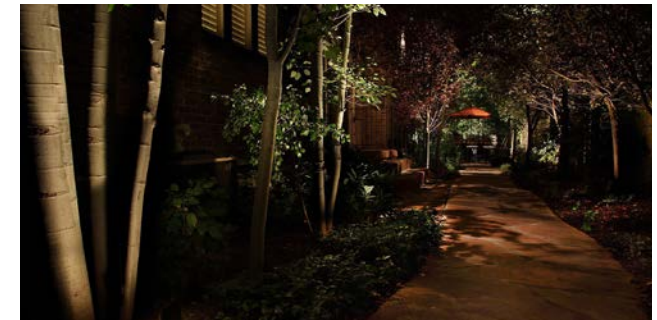
Figure 61: Example of down lighting with bullet-type fixture placed above eye-level above trees to illuminate pathways.
