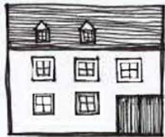
Loft conversion incorporating gabled dormers.
